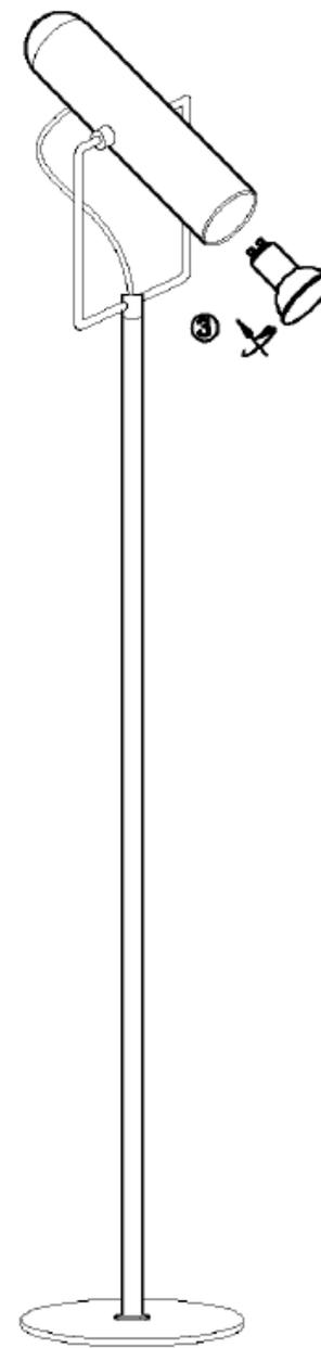
Assemble a new GU10 led bulb
